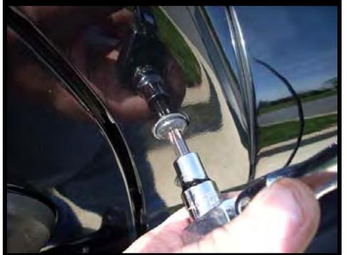
**Step 3:** Remove the front 2 torx head bolts from the windshield retainer bracket.
